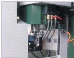
Protected automatic toolchanger
